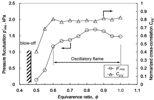
Fig. 4. Effect of equivalence ratio on pressure fluctuations and normalized cross-correlation
