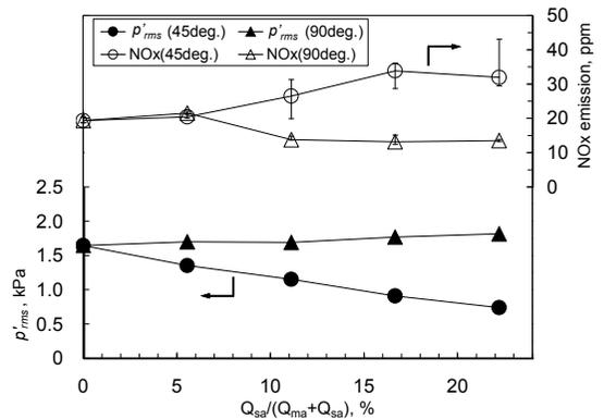
Fig. 10. Effect of SAI on  $p'_{rms}$  and NOx emissions
