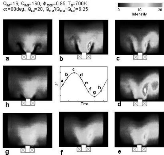
Fig. 11. 11B OH-PLIF images for non-effective case ( $\alpha=90\text{deg.}, Q_{s_a}/Q_{m_a}+Q_{s_a}=6.25\%$ )
