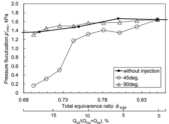
Fig. 12. Effect of SAI on pressure fluctuations
