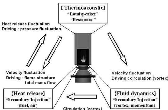
Fig. 1. Schematic image of dominant factors on oscillatory combustion
