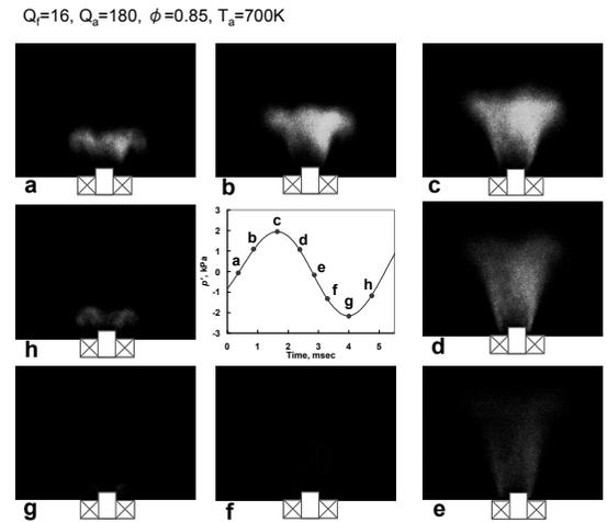
Fig. 7. Phase-locked OH\* chemiluminescence images of the self-excited oscillation (average of 100 images)
