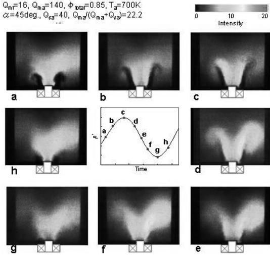
Fig. 11. 11A OH-PLIF images for effective case ( $\alpha=45\text{deg.}, Q_{s_a}/Q_{m_a}+Q_{s_a}=22.2\%$ )
