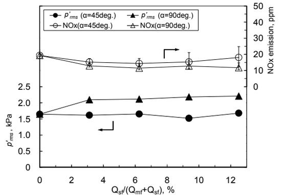
Fig. 9. Effect of SFI on  $p'_{rms}$  and NOx emissions
