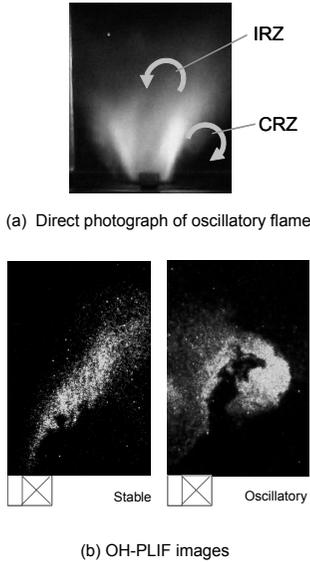
Fig. 8. Flame characteristics: (a) direct photograph of the oscillatory flame, (b) OH-PLIF images
