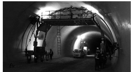
Fig.12 Overview of an actual tunnel inspection system
