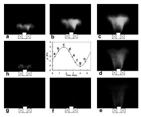
Fig. 7. Phase-locked OH\* chemiluminescence images of the self-excited oscillation (average of 100 images)
