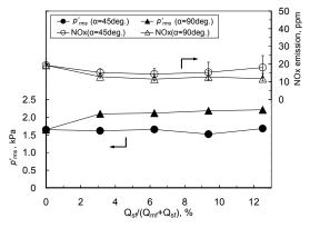
Fig. 9. Effect of SFI on  $p'_{rms}$  and NOx emissions
