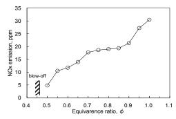
Fig. 5. Effect of equivalence ratio on NOx emissions
