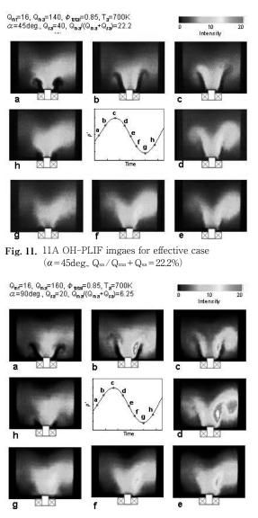
Fig. 11. 11B OH-PLIF images for non-effective case  $(\alpha = 90 \text{deg.}, Q_{\text{sa}} / Q_{\text{ma}} + Q_{\text{sa}} = 6.25\%)$
