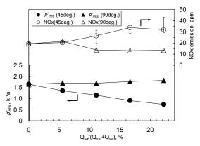
Fig. 10. Effect of SAI on p'rms and NOx emissions
