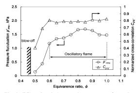
Fig. 4. Effect of equivalence ratio on pressure fluctuations and normalized cross-correlation
