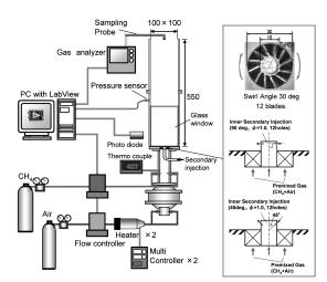
Fig. 2. Experimental setup
