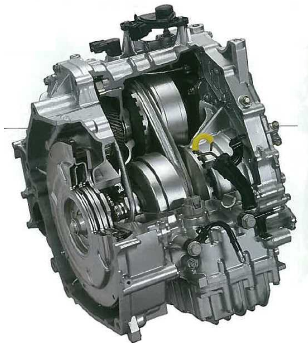
図 1.3 CVT (Continuously Variable Transmission) の機構
