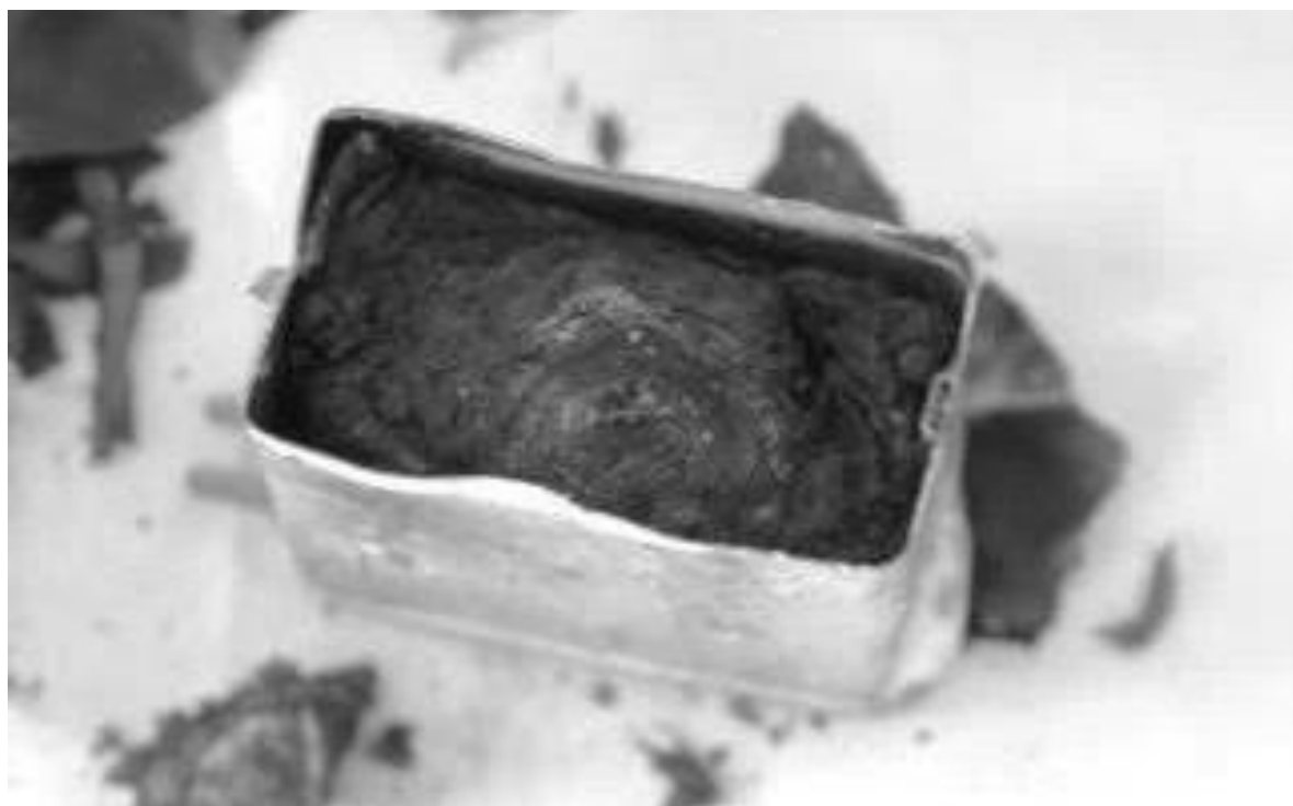
Figure 16. Inside a capacitor after the inductive heating treatment (reference)
