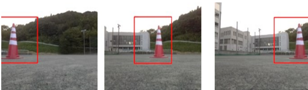
Fig. 3-2-2 Three-part image classification to determine left/right
